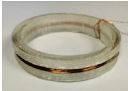
50-turn enameled copper coil, with conductor radius 0.15 mm, cover thickness 0.03 mm.
