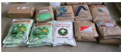
Cold asphalt mixture
