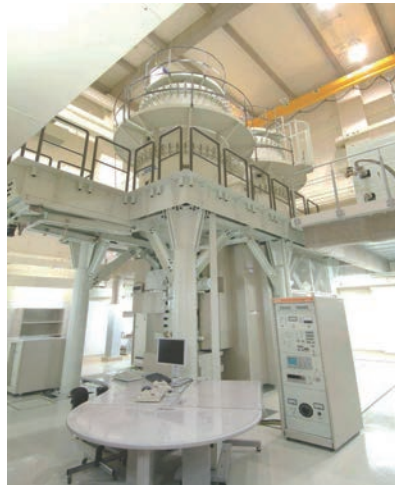
JEM-1300NEF with \Omega energy filter
