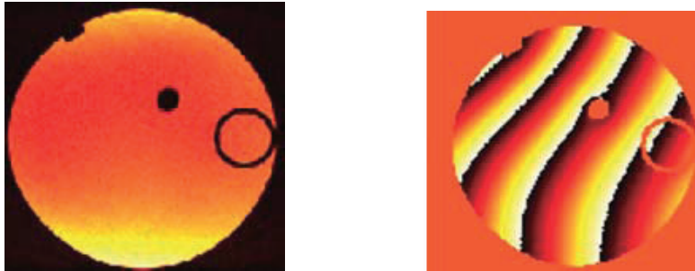
Figure : M_{\pm}(x, y, z_0) = M(x, y, z_0) \exp(\pm i\gamma B_z(x, y, z_0)T + i\varphi_0)
