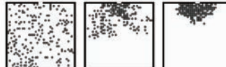
Fig. 3. People leaving a room with one door only. Displayed are three typical stages of the dynamics.
