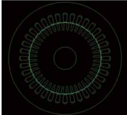
Fig. 12. A rotating machine model with an air gap
