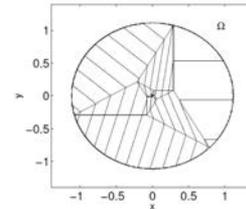
b) Numerical computation of a 2-dim stochastic microstructure.
