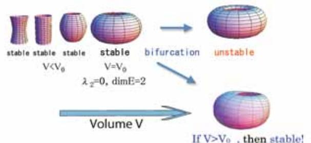
Fig. 2: Equilibrium surfaces of area with volume constraint spanned by two coaxial circles with the same radius. Stable solutions can have lower symmetry than unstable solutions.
